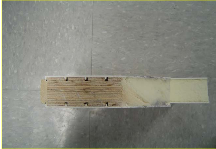
Leaf Cross Section at Lock Stile
