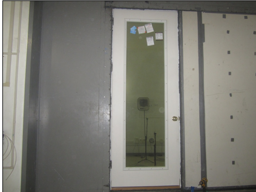
Receive Room View of Installed Specimen
